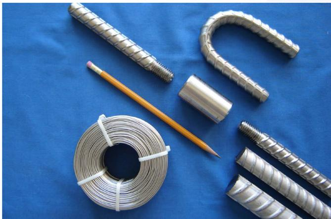
Stainless steel components for concrete reinforcing: rebar, U-bent rebar, threaded rebar, tie-wire and rebar coupler. (Photo Courtesy of F. N. Smith)
