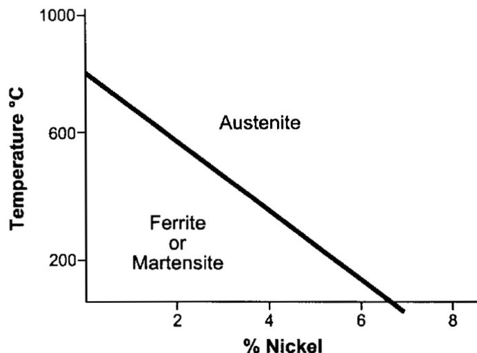
11-14%, corrosion is practically negligible in the atmosphere. Nickel in stainless steel promotes austenite stability and reduces the temperature at which austenite can exist. *Figure 3* illustrates this effect. Above the diagonal line in the diagram, austenite is stable at the indicated temperature; below the line, either ferrite or martensite is the stable crystal structure.
