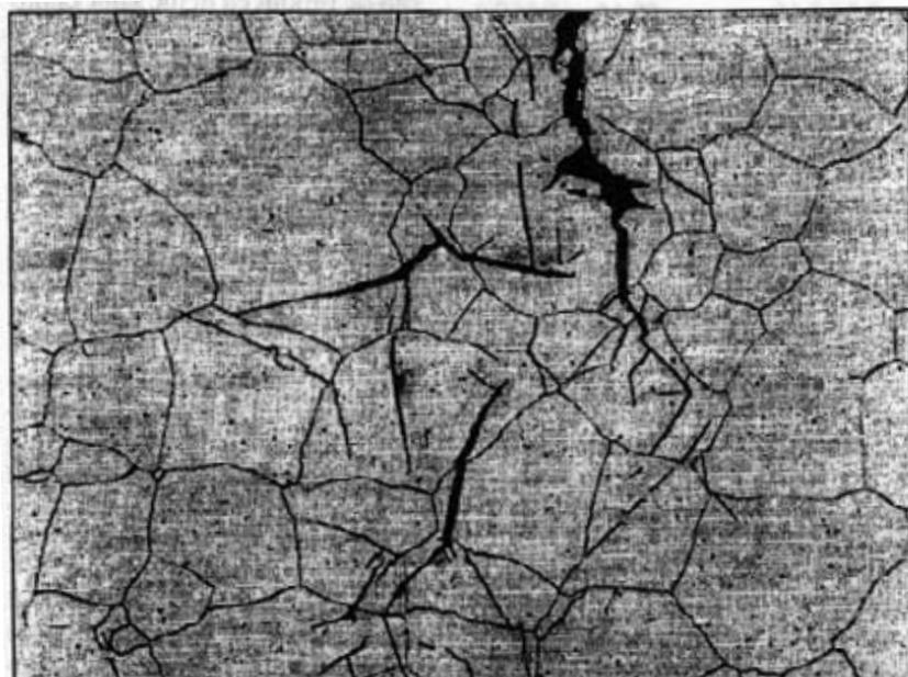
in ammoniacal environments and carbon and alloy steels, including stainless steels, in strongly alkaline solutions. Chloride stress corrosion cracking, the most common form of environmentally induced cracking in austenitic stainless steels, requires the presence of chloride ions, tensile stresses, and elevated tempera-
