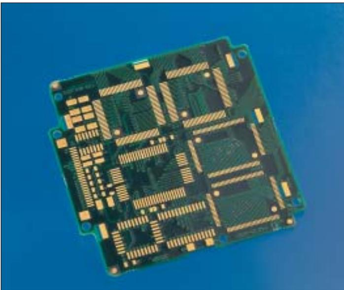
**Figure 26** Electroless nickel/immersion gold deposits offer many advantages in printed circuit board production.
