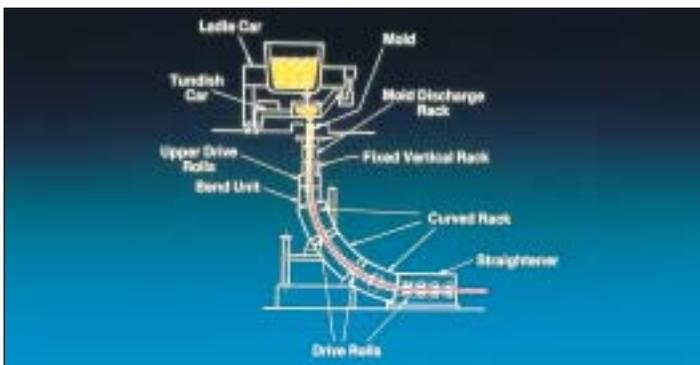
**Figure 14** Continuous casting of semi-finished steel products.
