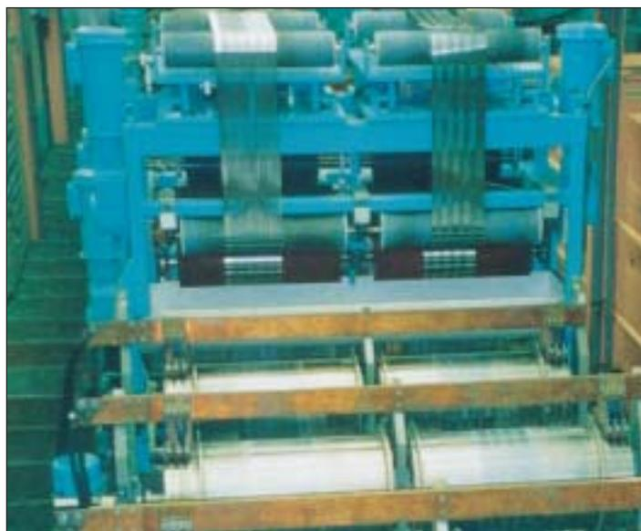
**Figure 22** Continuous nickel plating of perforated steel strip for use as a substrate in the production of sintered nickel electrodes.
