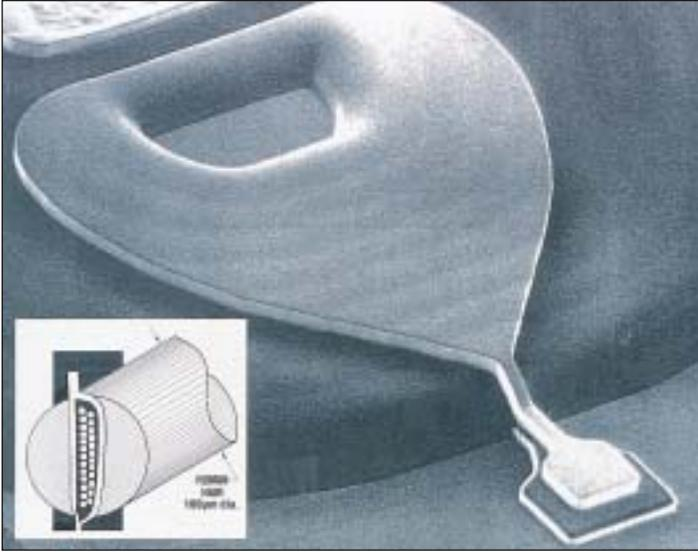
**Figure 6** An electroformed thin film inductive head and a cross section comparing size with a human hair.
