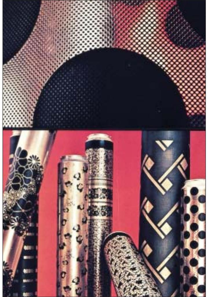
**Figure 38** Typical electroformed rotary screens with patterns applied by photoresist techniques. Close-up shows sealed areas and open areas through which dye can flow.
