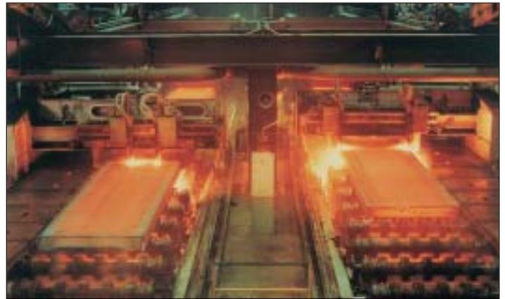
**Figure 15** Continuous steel casting being cut into slabs ready for hot rolling.
