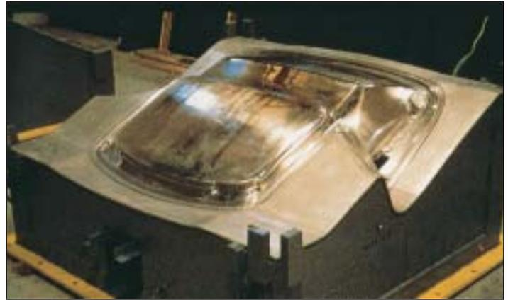
**Figure 12** Electroformed nickel mold for reinforced plastic automotive body component.
