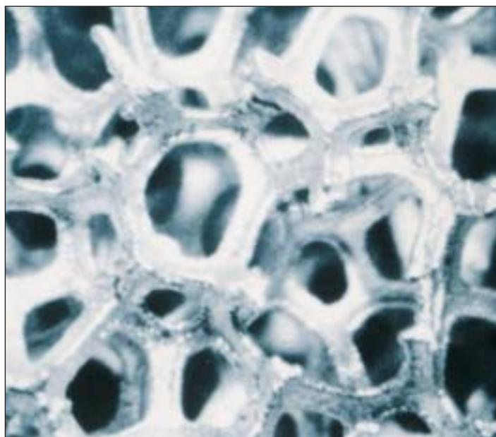
**Figure 24** The high porosity skeletal structure of electroformed nickel foam.
