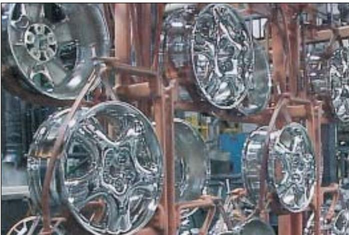
**Figure 8** Popular plated aluminum wheels offer style, excellent corrosion resistance, lightweight and recyclability. (Courtesy of Kuntz Electroplating Inc.)
