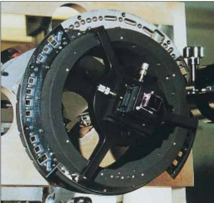
**Figure 32** Critical components on the Space Telescope Imaging Spectrograph (STIS) used on the Hubble Space Telescope (HST) are made by electroforming.
