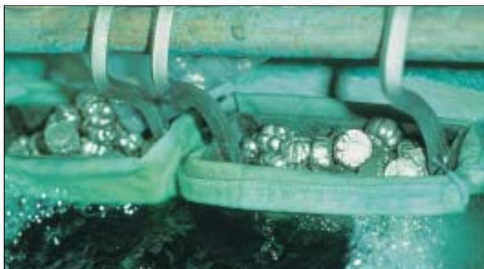
**Figure 1** Nickel units are provided by soluble salts and nickel metal in titanium baskets.
