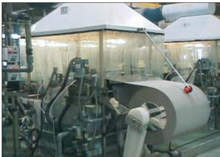
**Figure 23** Nickel foam is coiled after continuous electroforming operation.
