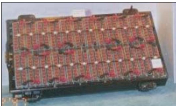
**Figure 21** Typical Ni/MH battery pack for electric cars.
