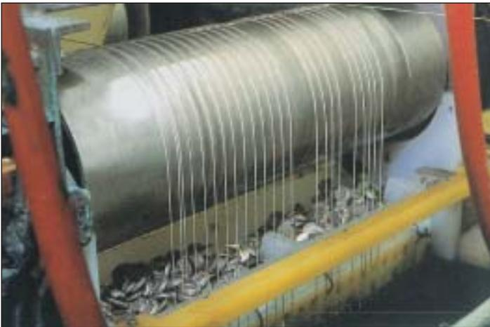
**Figure 27** Continuous nickel plating of heavy copper wire prior to being drawn down to fine, corrosion and heat resistant wire for critical applications
