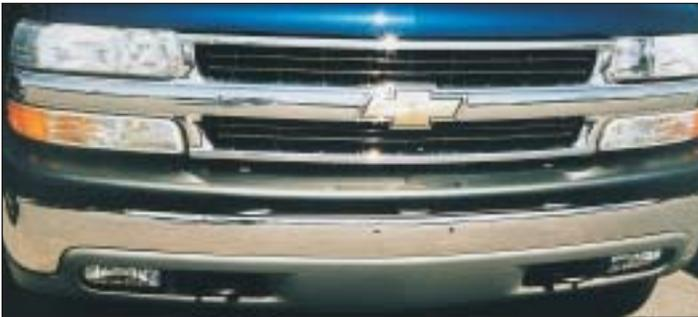
**Figure 7** Demand for plated steel bumpers has been strong. Parts have visual appeal, excellent durability and good recyclability.
