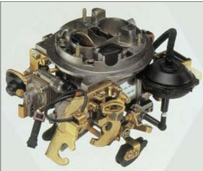
**Figure 10** Electroless nickel was required to resolve corrosion problems on carburetors using ethanol fuel.
