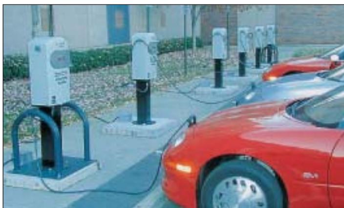
**Figure 20** Recharging an electric car powered by Ni/MH batteries.
