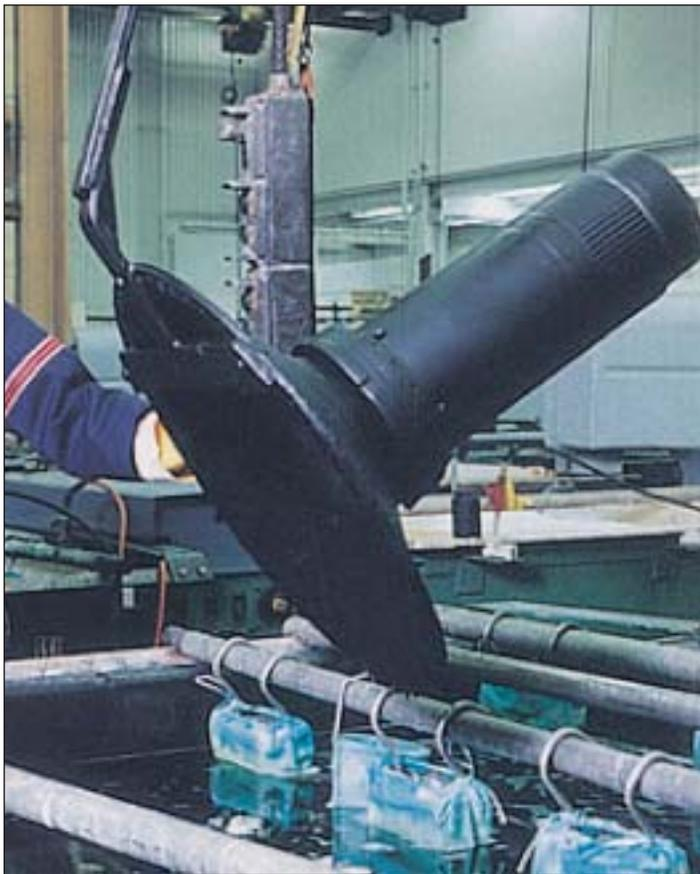
**Figure 29** Heavily masked CF-6 hub is nickel plated to repair a damaged or over-machined area..
