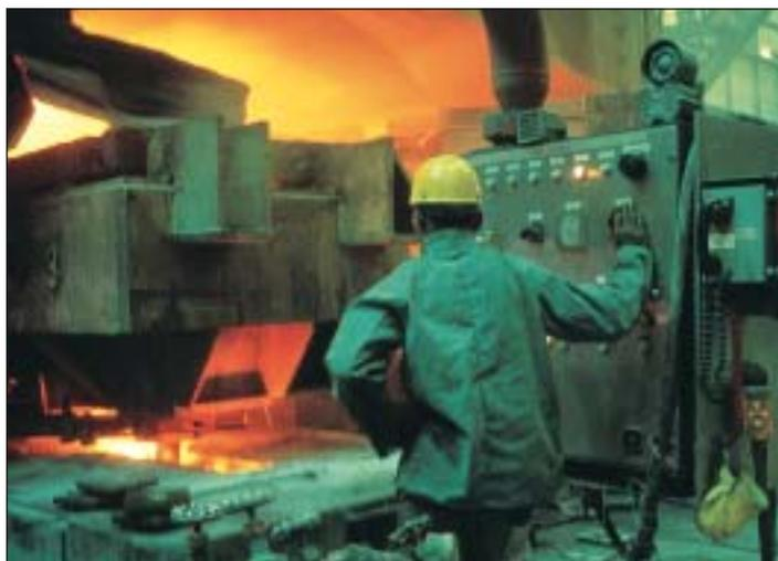
**Figure 17** Aggressive conditions for nickel plate at the molten steel casting station.
