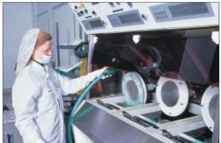
**Figure 3** CD electroforming station. Nickel stampers being rinsed over tank prevents solution loss. (Courtesy of Sony Music Canada)
