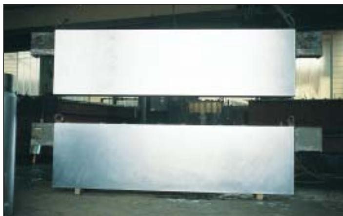
**Figure 18** A pair of nickel plated side plates for a huge mold.
