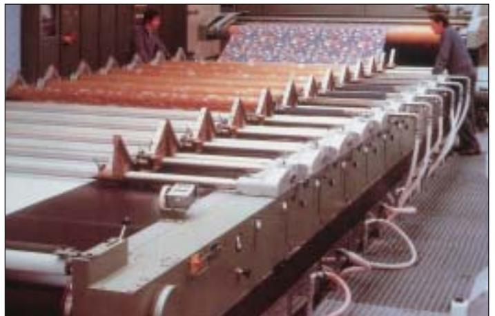
**Figure 39** Textile printing machine using electroformed nickel screens.
