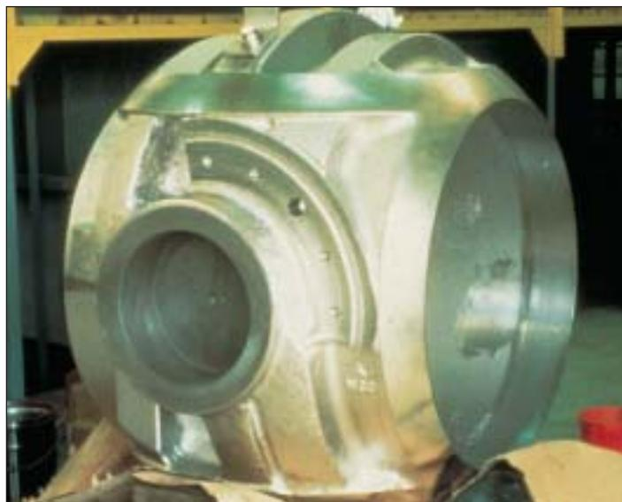
**Figure 36** Electroless nickel plated ball valve plug, 105 cm diameter. Thickness uniformity and corrosion resistance are major requirements of the deposit.
