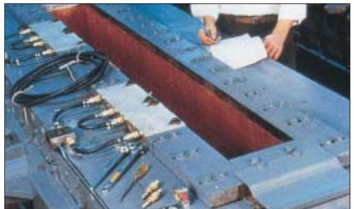
**Figure 16** A typical copper mold for continuous casting of steel.
