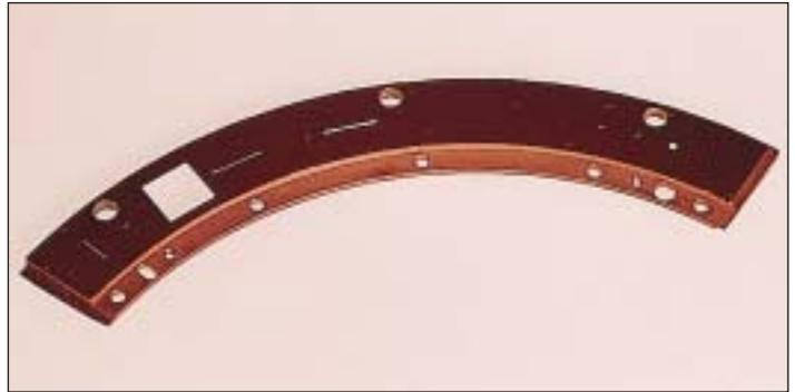
**Figure 33** One of four high precision, electroformed nickel slit wheel segments essential to the success of the STIS and the HST.
