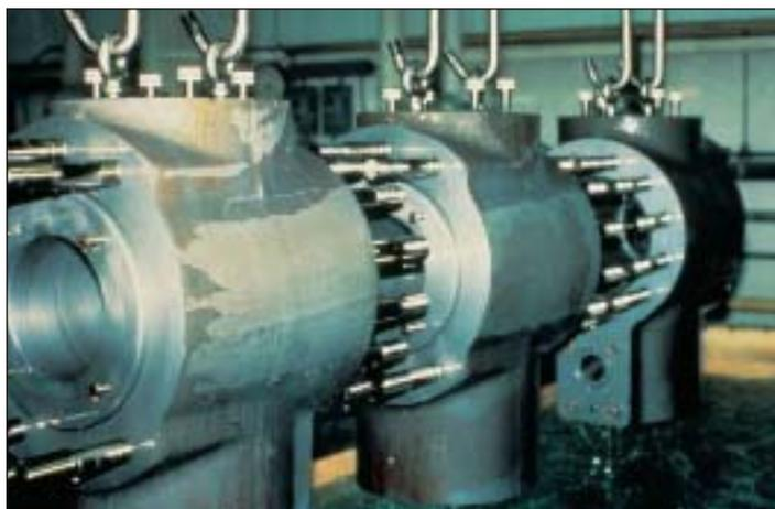
**Figure 35** Electroless nickel plated mud pump bodies.
