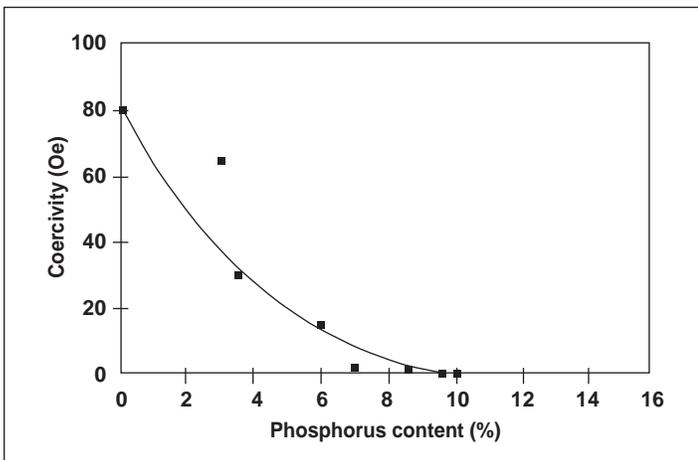
**Figure 4** Effect of phosphorus content on magnetic properties of electroless nickel.
