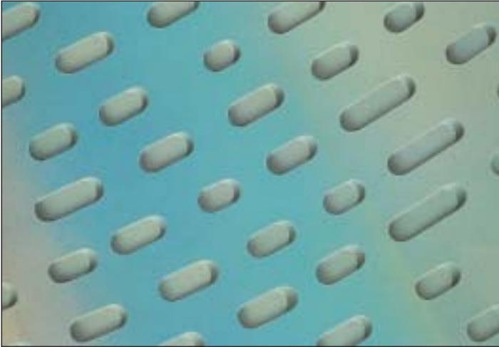
**Figure 2** Spiral pattern of submicron pits on CD surface. Perfect replication depends on nickel electroforming.
