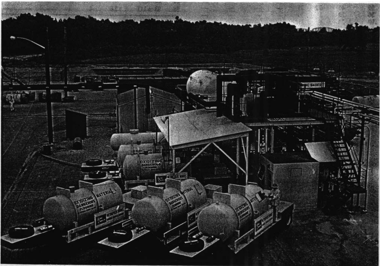
Fig. 3 - ICC-authorized tanks for bulk shipments of liquid fluorine. Each loss-free, Dewar-type tank consists of three concentric shells and heads. The highly corrosive fluorine is contained in an inner shell of nickel-copper alloy 400.
