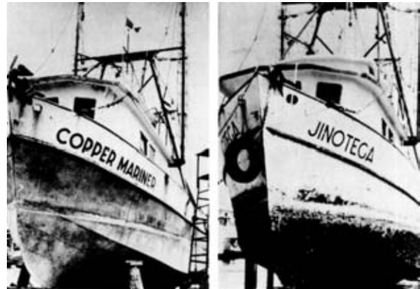
Comparison of fouling of copper-nickel hull of "Copper Mariner" with steel hull of sister ship "Jinotega". (INCO (Europe) Ltd)
