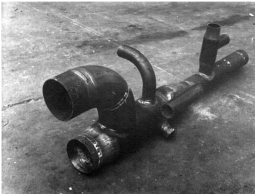
Illustrating the use of a variety of fabrication procedures. This 90/10 copper-nickel prefabricated pipework assembly shows swaged reducers, small radius bends and butt welds. Pipe sizes are from 75 to 200 mm nominal bore. (Vickers Shipbuilding & Engineering Ltd)
