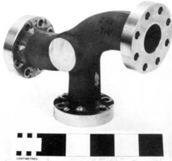
A complex casting in the proprietary 70/30 type copper-nickel-chromium alloy IN 768 produced for the Ministry of Defence by the BNF Metals Technology Centre.
