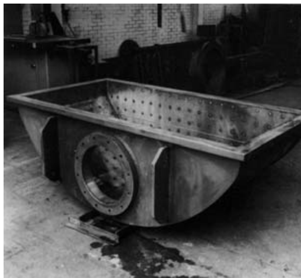
A water box used to collect and distribute water from and to bundles of tubes in one stage of a desalination plant. Because of the turbulent water flow expected, the steel casing has been lined with copper-nickel sheet by spot welding. (Portobello Fabricators Ltd)
