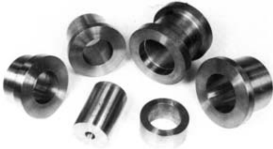
Typical forged and machined components in 70/30 copper-nickel for use in seawater systems. Flange diameters are over 300 mm and piece-weights as forged from 28 to 184 kg. (Doncaster Special Alloys Products Ltd)
