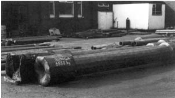
A large forging weighing 6,550 kg in 70/30 copper nickel. (N. C. Ashton Ltd)
