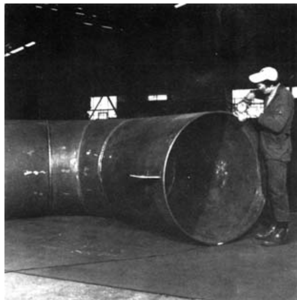
A welded 90/10 copper-nickel pipe 1420 mm outside diameter for use in the Dubai desalination plant brine recirculation system. (Yorkshire Imperial Alloys)
