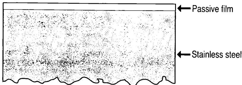
Figure 1. Cross-section of stainless steel surface.
