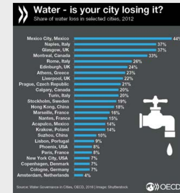
Figure 1: Leakage rate in major cities Source: OECD (Water Governance in Cities, 2014) - Shutterstock
