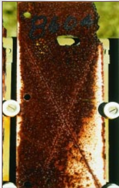
Painted cold rolled steel exposed since 1988.
