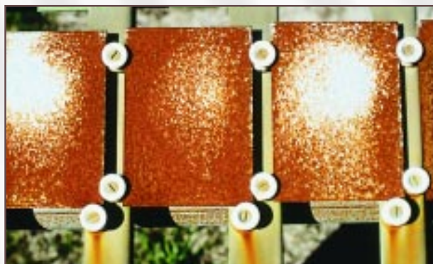
Bare G-90 galvanized steel exposed since 1981.
