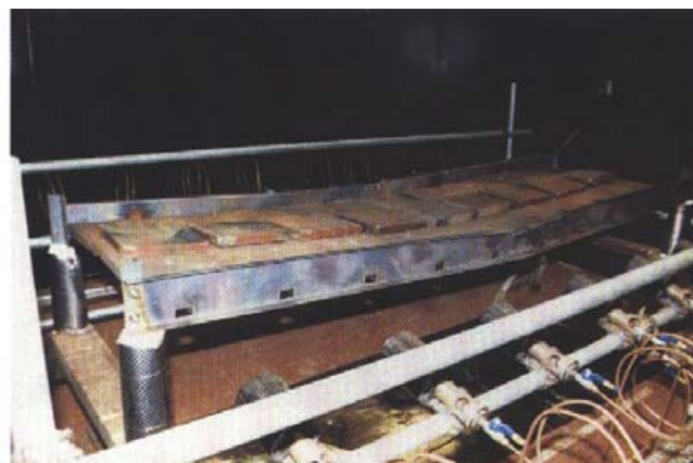
Bottom right: Stainless steel ladder after fire resistance test (extended to 45 minutes, see text). Structural integrity was maintained throughout test and central deflection was only 80.5 mm at conclusion.
