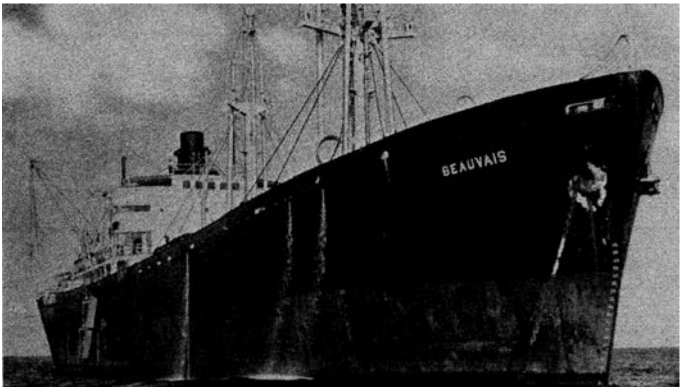
Figure P Experimental tanker Beauvais , rebuilt in 1960-61 by Gaz Transport to test several designs of cargo tanks.
