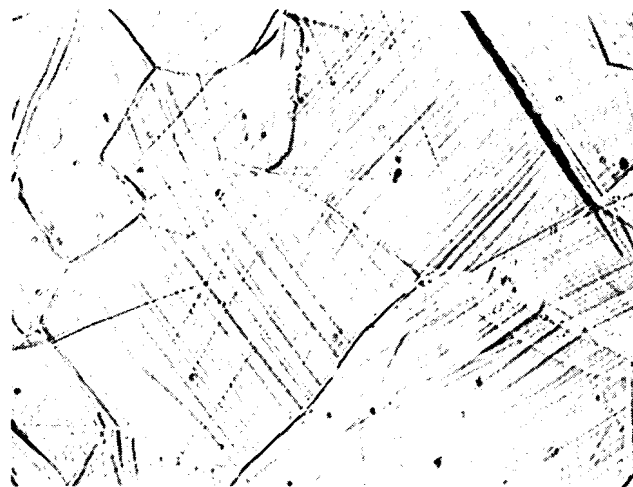
Surface slip traces on chemically polished iron sheet tensile specimen strained 5 pct at -320F (-196C) . Slip traces are planar and restricted to one type of slip system. Magnification 175 times.
