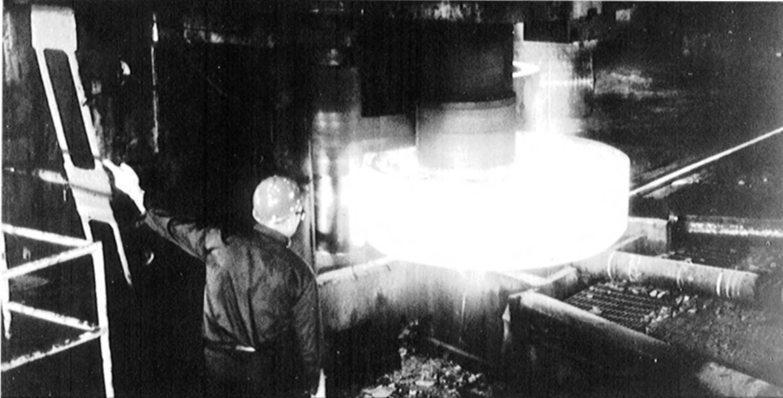
Figure 8—Large forgings, 26"—600 lb weld neck flanges of IN-787 were used in the Alyeska oil line because of the excellent combination of strength and low temperature notch toughness. The section thicknesses ranged from 2¼" to 7½".
