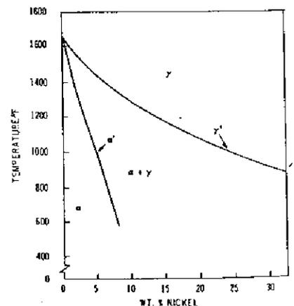
Fig. 4—Iron-nickel equilibrium diagram (after Owen and Liu)
