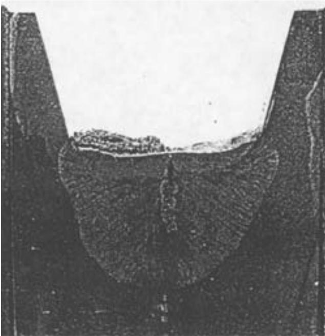
Fig. 43—Centerline cracking in the first pass of a submerged-arc weld in 18Ni (250) maraging steel. Etchant: Lepito's Reagent. X3 (Reduced 15%)
