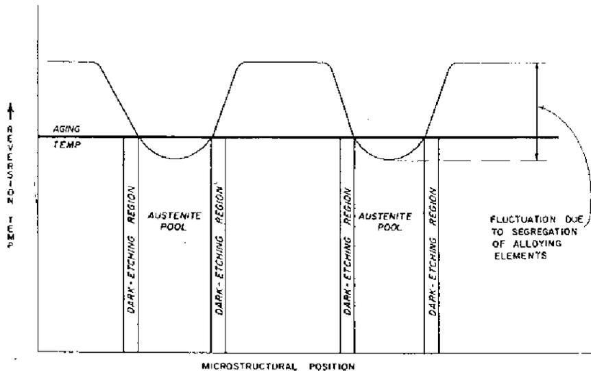
Fig. 33—Schematic illustration of austenite pool formation
