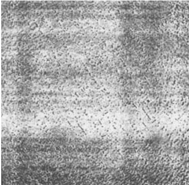
Fig. 45—Photomicrograph of submerged-arc deposit in 18Ni (250) showing extent of inclusions present. As-polished. X 100
