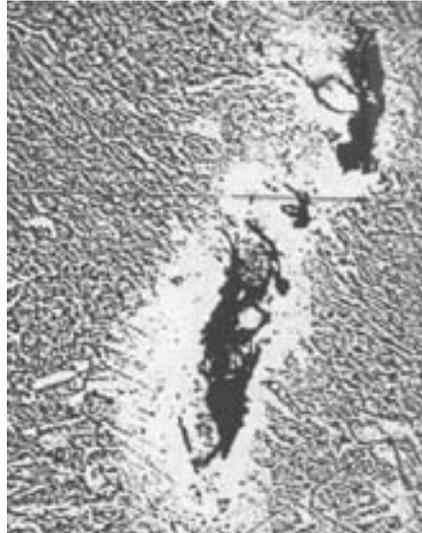
**Fig. 19—Cracks and voids in austenite pools ahead of a propagating crack. (a) optical micrograph, X750 (reduced 40%) (b) parlodian replica, X7000 (reduced 40%). Etchant: modified Fry's Reagent**
