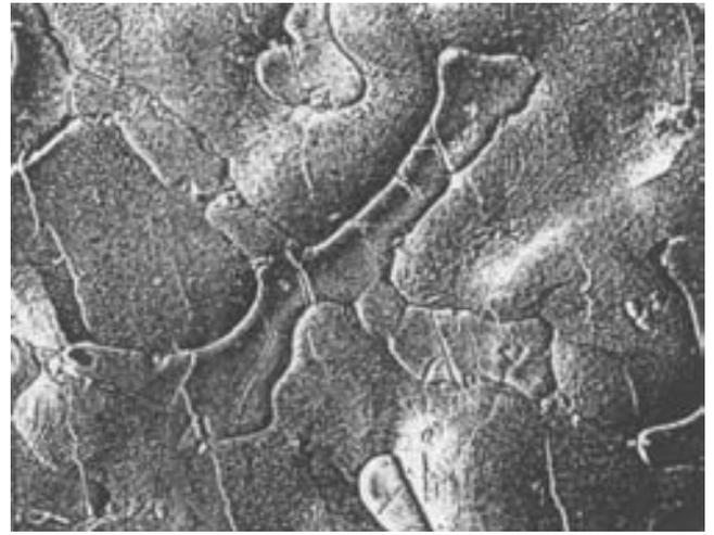
Fig. 44—Electron micrograph of fracture face of centerline crack in a submerged-arc weld in 18Ni (250) showing extent of brittle films. X6000 (Reduced 60%)
