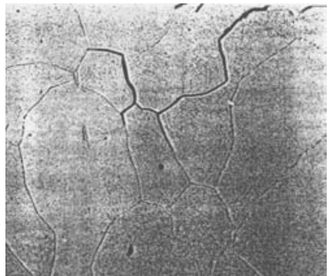
Fig. 50—Cracks along the grain boundaries in the heat-affected zone of a submerged-arc weld. Note the grain boundary particles. Etchant: modified Fry's Reagent. X750 (Reduced 15%)
