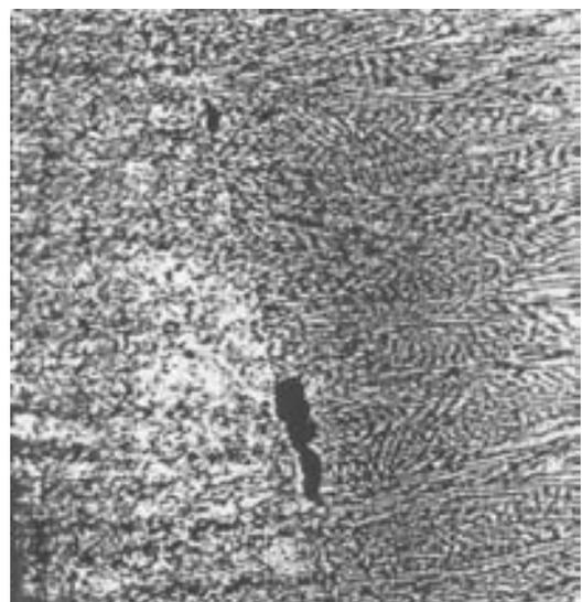
Fig. 54—Secondary cracks in weld metal close to fusion boundary, etched in 5% nital. X 150
