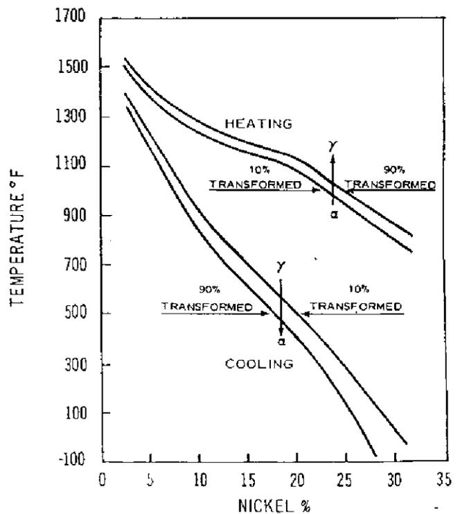
**Fig. 1—Iron-nickel transformation diagram (after Jones and Pumphry)**
