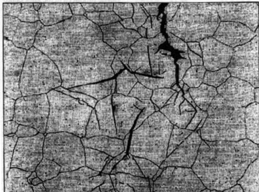
Figure 8. Transgranular chloride stress corrosion cracking of an austenitic stainless steel
