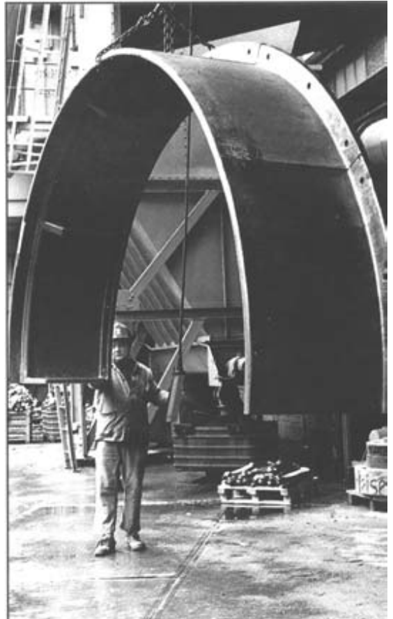
This is a side view of half of a rotary cement kiln entrance made from HD (GX40CrNiSi 27-4, 1.4823). It weighs 990-pounds (450 kg).
