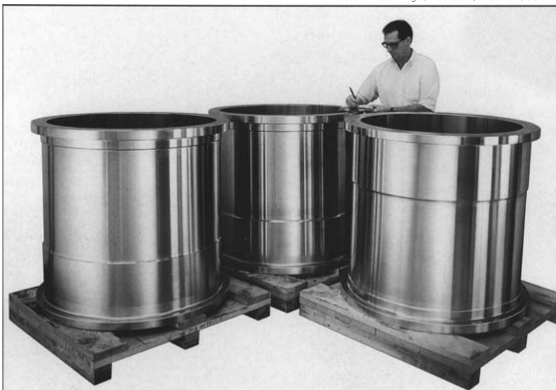
These are centrifugally cast CA15 turbine combustor cases.
