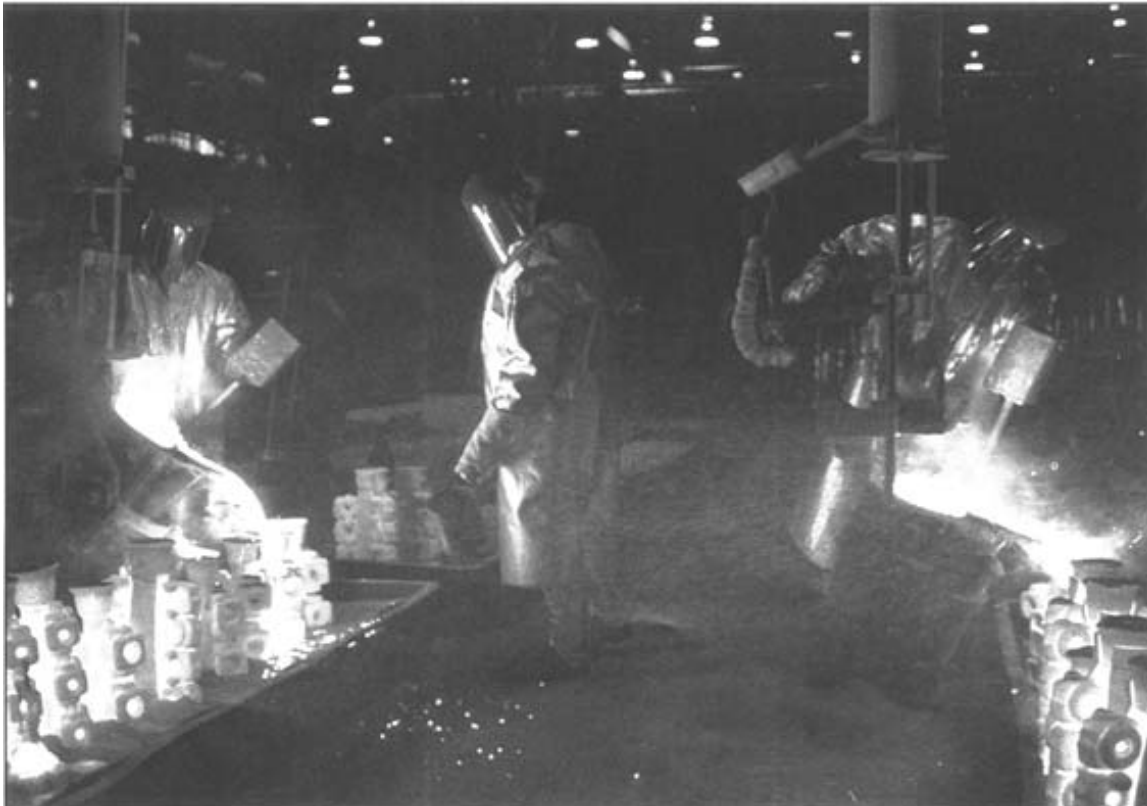
Pouring molten stainless steel into molds.
