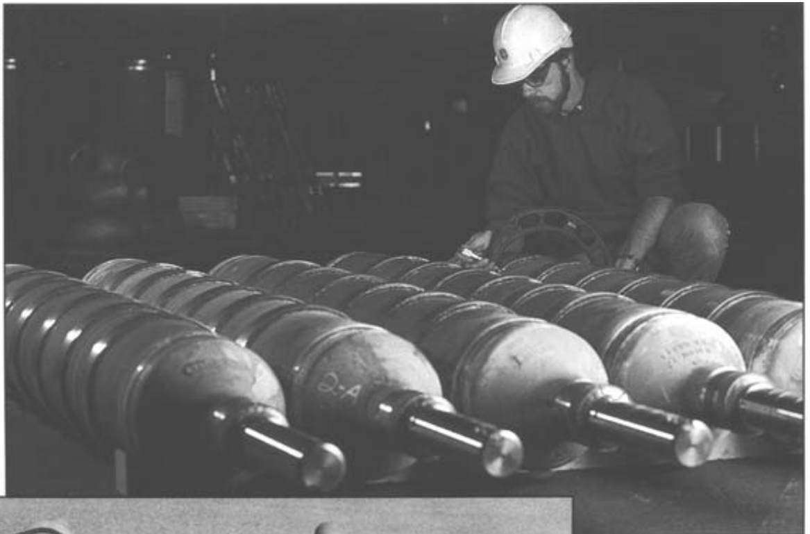
These slab reheat or "Tunnel" furnace rolls are made from Super 22H.
