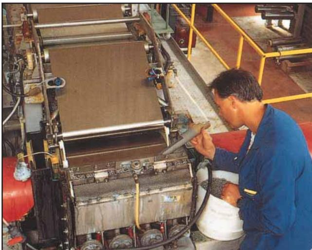
**Figure 15** Electroforming of nickel foil.
