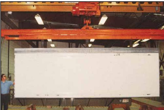
**Figure 8** Large nickel mould for compression moulding of hardboard panels.
