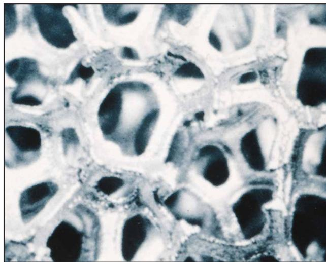
**Figure 16** The skeletal structure of electroformed nickel foam.
