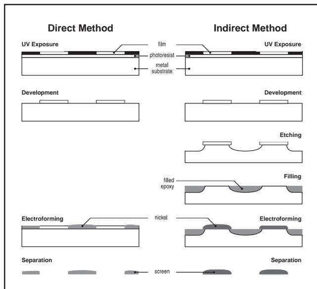
**Figure 2** Direct and indirect methods of producing screen patterns using photoresists.
