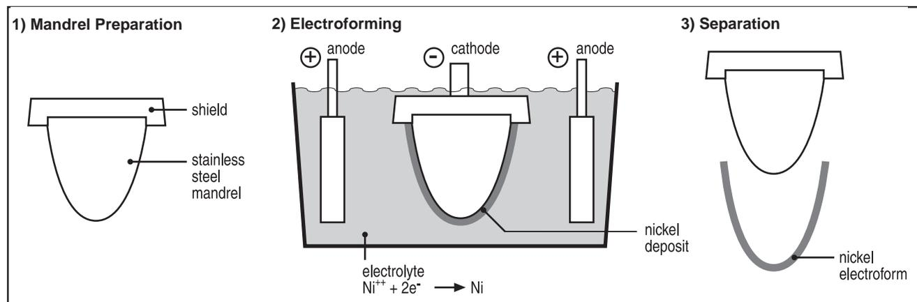
**Figure 1** Schematic of an electroforming operation.
