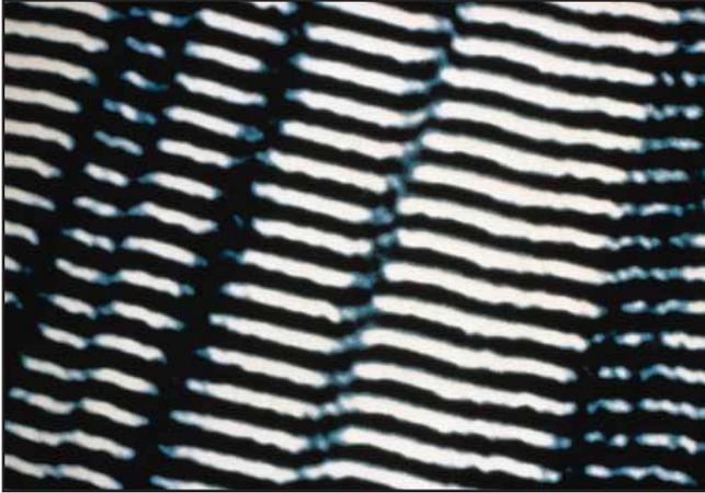
**Figure 10** Electroformed nickel embossing tools for holograms have a pattern of submicron grooves.
