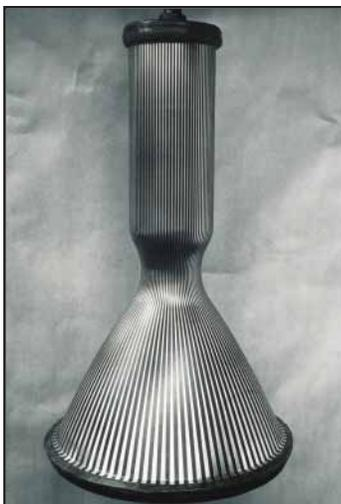
**Figure 13** Channels machined in the metal liner of a rocket thrust chamber, for the NASA Space Shuttle.
