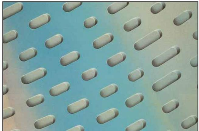
**Figure 9** Submicron pits on CD surface produce high quality sound. Perfect replication is dependent on nickel electroforming.
