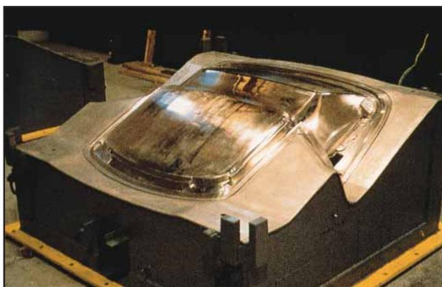
**Figure 7** Nickel mould for automotive body component.
