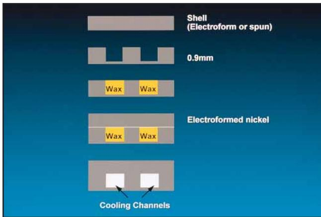
**Figure 12** Stages in the electroforming of internal passages.
