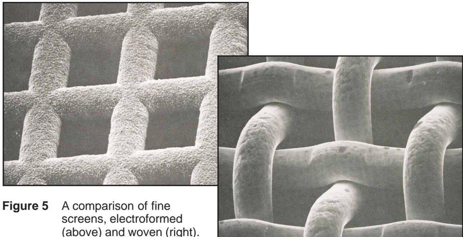
**Figure 5** A comparison of fine screens, electroformed (above) and woven (right).
