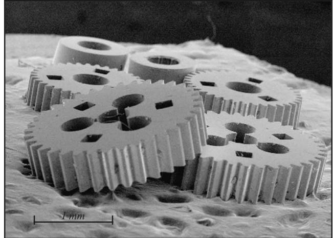
**Figure 17** Gears and spacers for micro-magnetic motor applications.
