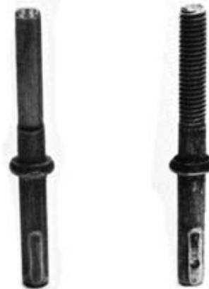
**Terminal Stud** Originally produced by machining, this electrical terminal stud is now cold headed of Type 430 stainless steel at 1/3 the cost. The wafer-thin collar is upset with two flats that prevent its turning in an insulator. The top half of the shank is extruded, also with two flats, and the threaded end is extruded. Secondary operations include roll-threading and drilling of the top shank where a Nichrome wire is resistance welded.
