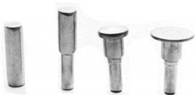
Typical stainless steel part produced by combining extrusion and upsetting on a multiple die forming machine. Extrusion reduces the diameter of the initial stock while increasing its length, and upsetting increases diameter and decreases length.
