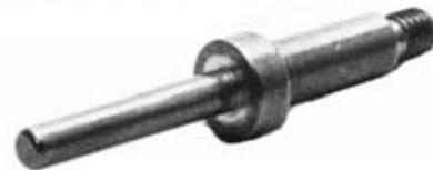
Disc spindle for water meter (formerly screw machined)—
