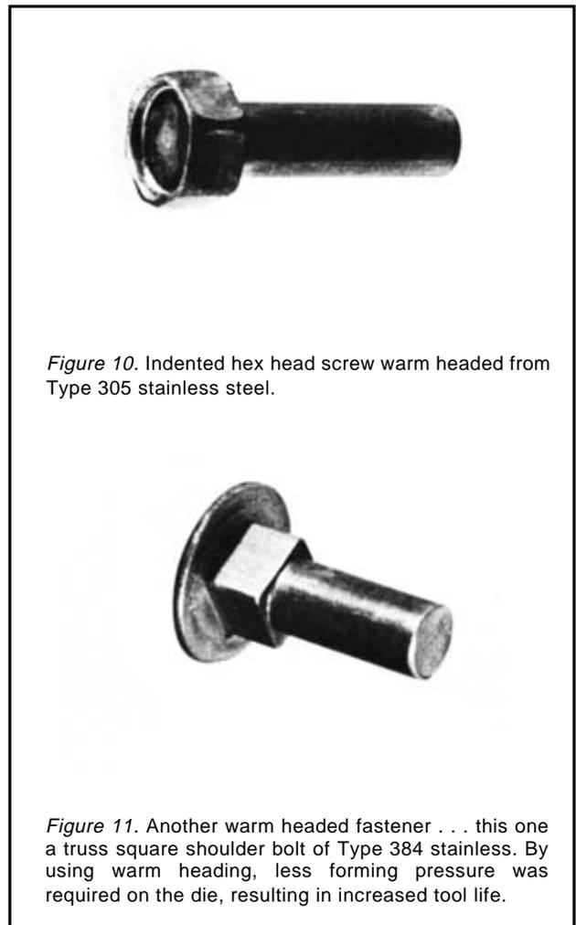
The result is that less pressure is required to fill the die cavity, sharper corners and shoulders are achieved, and the possibility of cracking is minimized. The accompanying illustrations in Figures 10 and 11 show examples of the improved forming made possible by warm heading techniques.
