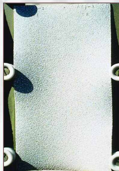
Pure zinc exposed since 1960 about 25 m (82 ft) from the mean high tide.
