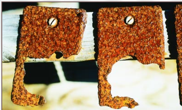
Coated (60 Zn, 20 Al, 20 Mg) carbon steel exposed since 1952.
