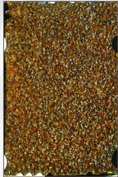
High strength low alloy weathering steel exposed since 1968.
