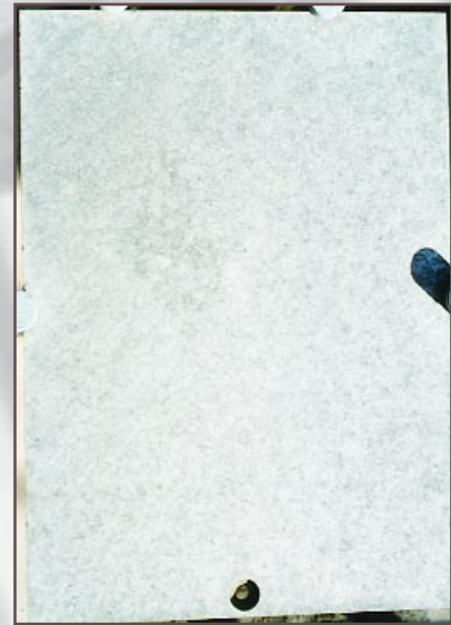
Aluminum alloy 6061 exposed since 1982 about 25 m (82 ft) from the mean high tide.
