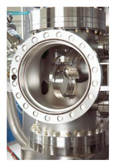
Welded equipment such as this vacuum chamber involving different product forms, a wide variety of metal thicknesses, and a highly polished surface finish is most easily produced using 300 series austenitic stainless steels.
