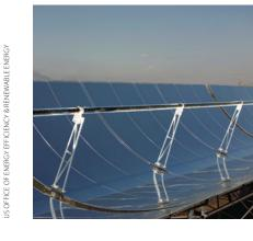
The parabolic trough system employs reflectors that focus solar radiation onto a fluid-filled receiver tube, concentrating it by a factor of about 100.
