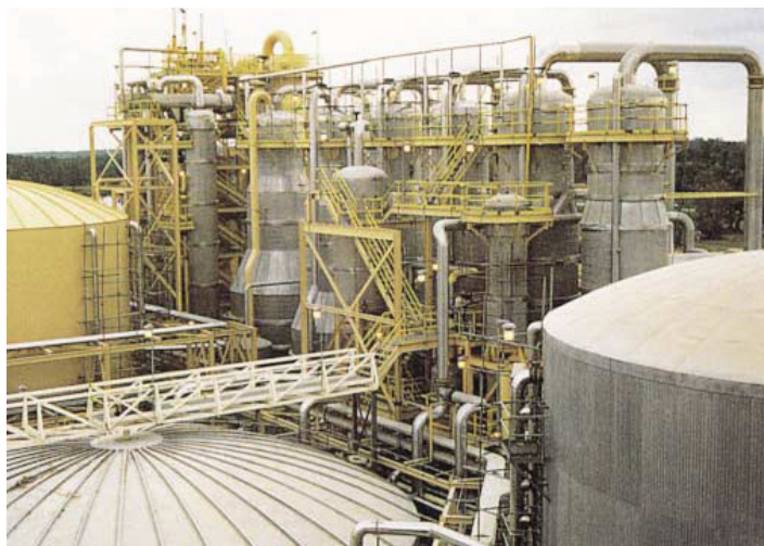
Figure 5-5 Evaporator train with foul condensate stripper and soap skim tanks
