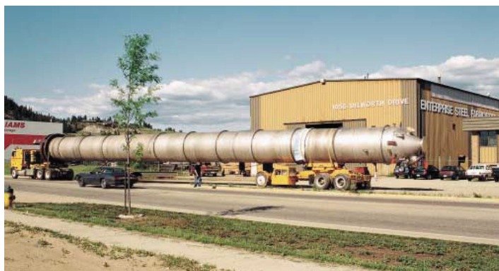
Figure 4-1 Alloy 2205 oxygen delignification vessel – Canada
