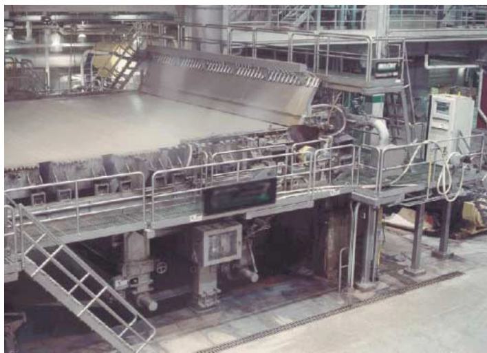
Figure 12-2 Fourdrinier wet end showing headbox
