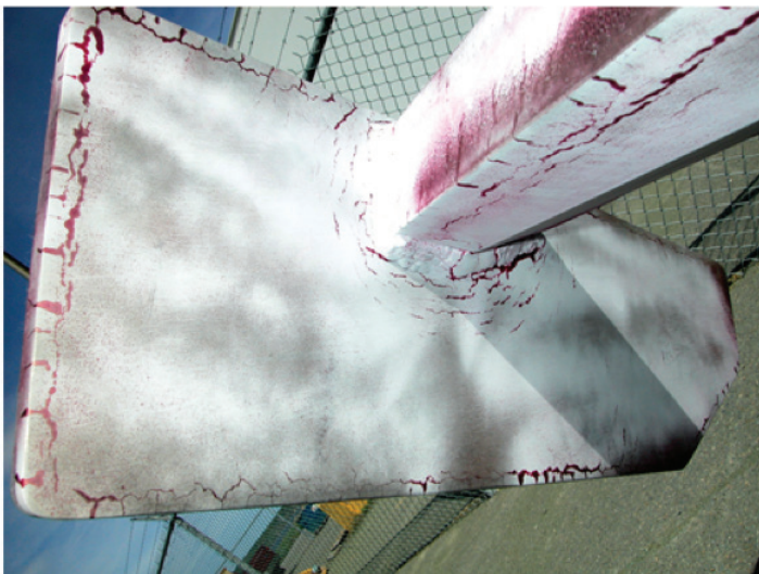
Figure 3-7 SCC of a solid Type 304L stainless steel scraper arm and end paddle after 11 months service
