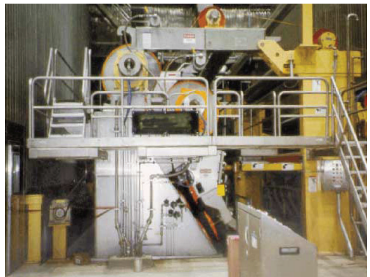
Figure 12-7 Typical size press
