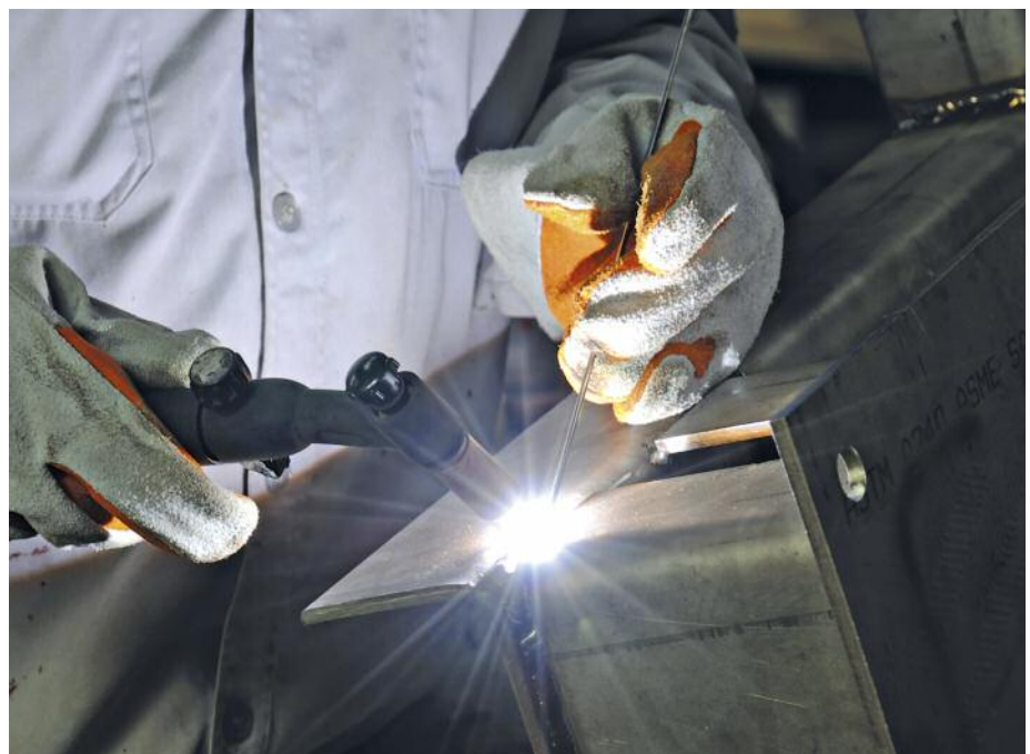
Manual GTA (TIG) welding. © iStock.com/Lekyum
