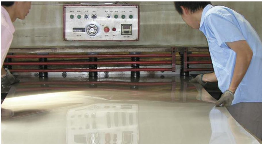
Shearing a stainless steel sheet. © IMO A
