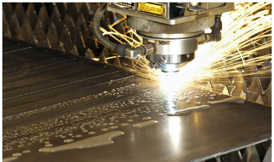
Rapid cutting of stainless steel sheet using a laser cutting process.
