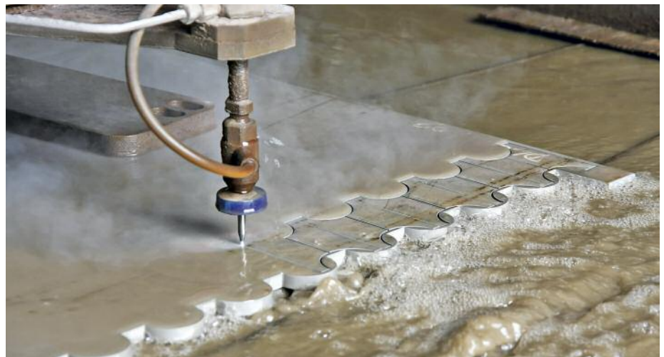
Water jet cutting of a stainless steel plate. © Lubos Chlubny/Shutterstock.com
