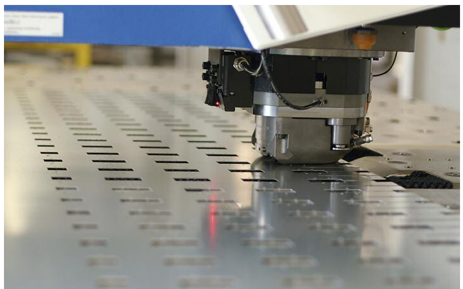
Piercing operation to produce a perforated stainless steel sheet.
