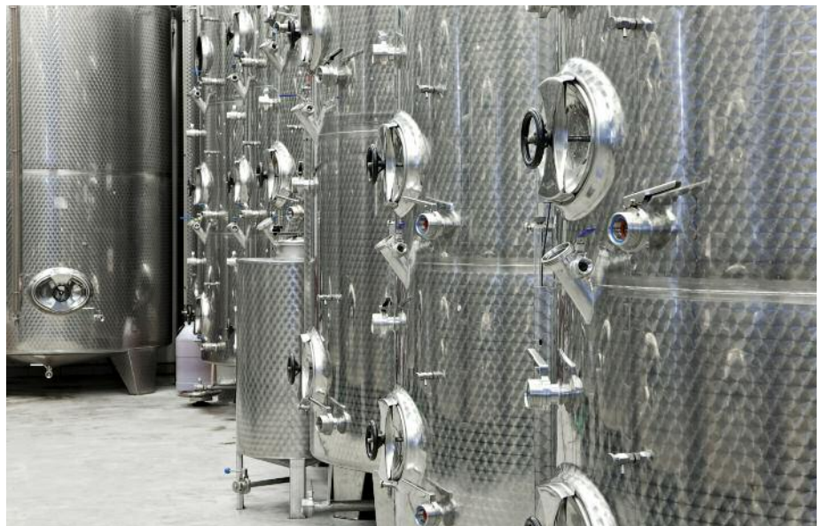
Wine tanks often use a fine, circular polished finish, which is hygienic, easy to clean, decorative and hides any dings and scratches. Surface finish requirements are an important part of the design process. © iStock.com/Josef Mohyla
