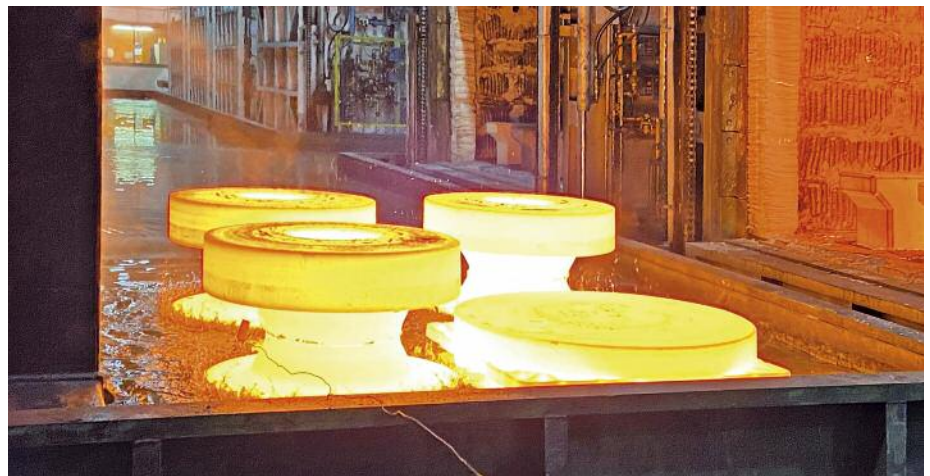
Water quenching of forged parts after they exit the solution annealing furnace. © Officine Ambrogio Melesi
