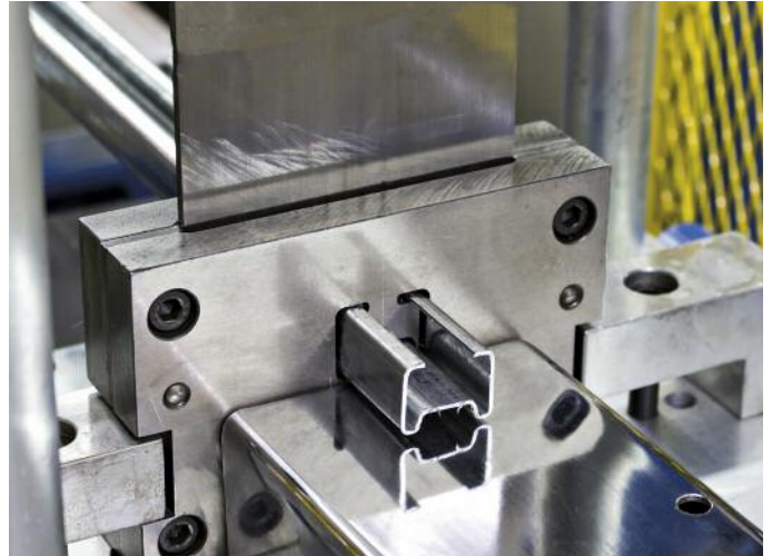
Formed stainless steel channel exiting a roll forming machine. © Warut Sintapanon/Dreamstime.com
