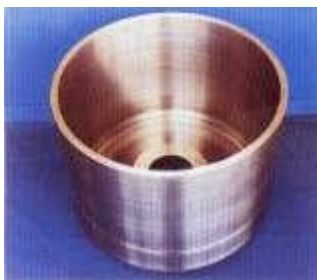
Figure 39. (DKI A 4358) Centrifuge body of G-CuNi30 (now CuNi30Fe1Mn1NbSi-C) for seawater desalination plant; cast and rough turned; weight approx. 250 kg
