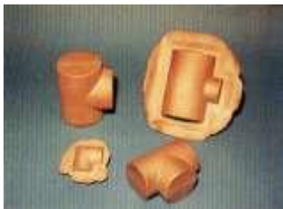
Figure 29. (DKI A 4980) Die forged parts of CuNi10Fe1Mn for manufacture of T and angle pieces for hydraulic systems in marine applications (weights: 0.8 to 2.9 kg)
