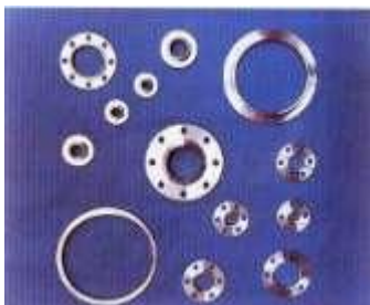
Figure 30. (DKI A 4354) Flanges of CuNi30Mn1Fe, weights 0.5 to 10 kg
