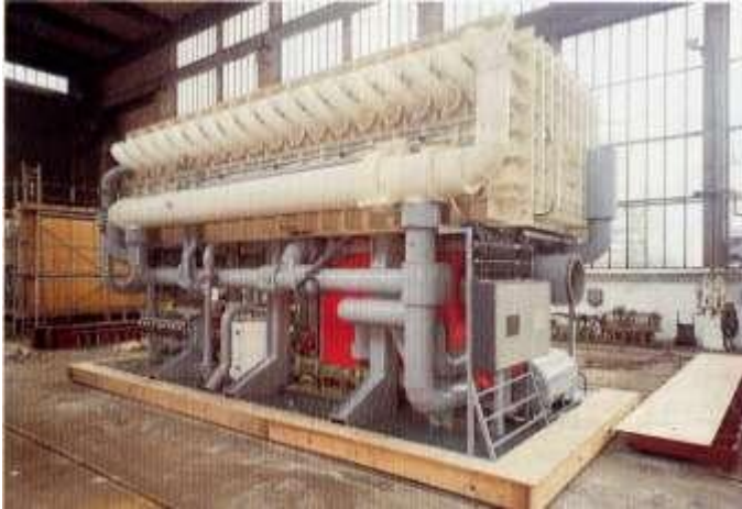
Figure 41. (DKI A 1221) Evaporator plant for fresh water production with an output of 500 m 3 /day. Condenser tubes, tubes of final heater, partition walls, housing, distillate troughs; all lines through which seawater passes and other important parts of the evaporator consist of CuNi10Fe1Mn
