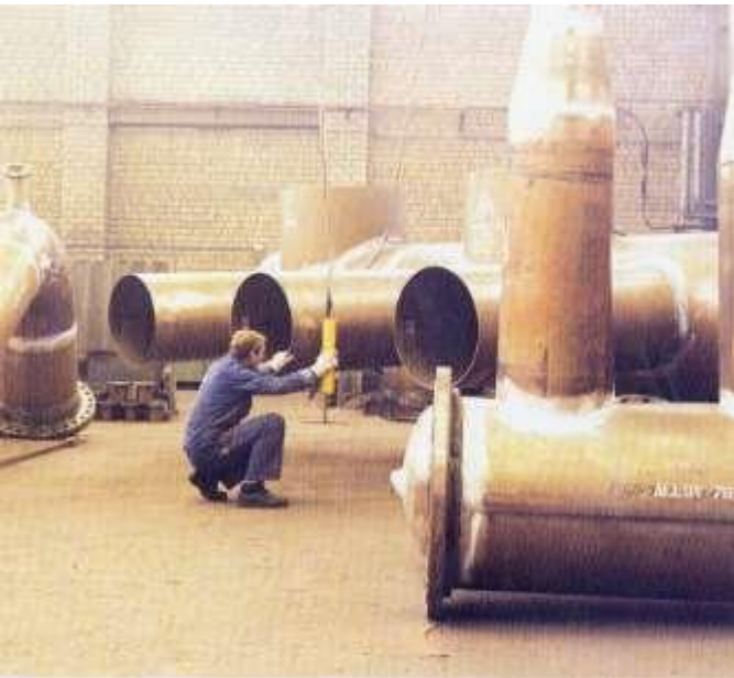
Figure 44. (DKI A 4975) Seawater piping system of Cu-Ni alloys for the YANBU seawater desalination plant in Saudi Arabia
