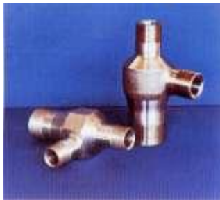
Figure 38. (DKI A 4356) T-piece of G-CuNi30 (now CuNi30Fe1Mn1NbSi-C) for high-pressure technology; cast and machined; weight approx. 40 kg
