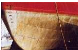
Figure 33(b). (DKI A 4893 and 4897) Hull of CuNi10Fe1Mn-clad sheet before launching (a) and after 2.5 months exposure in the Adriatic sea (b)
