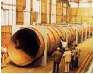
Figure 27. (DKI A 4970) Seawater inlet pipe for the firewater system of Jeddah airport in Saudi Arabia
