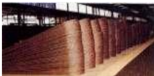
Figure 26. (DKI A 4969) Tube of CuNi10Fe1Mn; processed to tube bends, expandable (size: 17 x 1)
