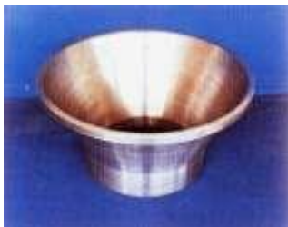
Figure 40. (DKI A 4359) Cone of G-CuNi30 (now CuNi30Fe1Mn1NbSi-C) for seawater desalination plant; cast and rough turned; weight approx. 110 kg
