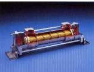
Figure 45. (DKI A 4976) Round tube heat exchanger for cooling oil, water, slow-burning liquid or emulsion by industrial, sea, river or brackish water; cooling tubes of Cu-Ni alloys
