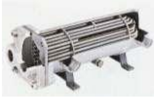
Figure 37. (DKI A 4217) Seawater and brackish water-resistant tube bundle oil heat exchanger for ship's gearbox. Seawater flows into the shell space and around the tubes. Gear oil flows through the tubes. Tubeplates, tubes (8 x 1 mm), deflector plates, shell with connection stubs and bottom flap valve consist of CuNi30Mn1Fe; overall length approx. 400 mm; dia. approx. 120 mm
