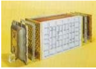
Figure 46. (DKI A 4977) Intercooler (water and air-cooled); cooling tubes of Cu-Ni alloys
