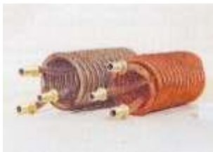
Figure 35. (DKI A 4087) Finned tube coils for hot water production in boilers and tanks; fin height 3.5 mm; materials Cu-Ni alloy containing 5% Ni (left) and SF-Cu
