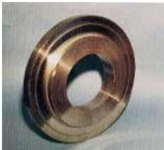
Figure 28. (DKI A 4979) Disc of CuNi14Al3 for manufacture of a compressor impeller, forged and rough turned (size: 450/150 mm dia., 80 mm thick)
