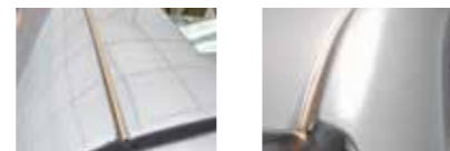
Laser-brazed roof seam on a Volkswagen Passat CC (2008)
