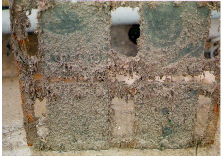
Fig 2 4 year exposure showing areas of brown slime removed after manual
