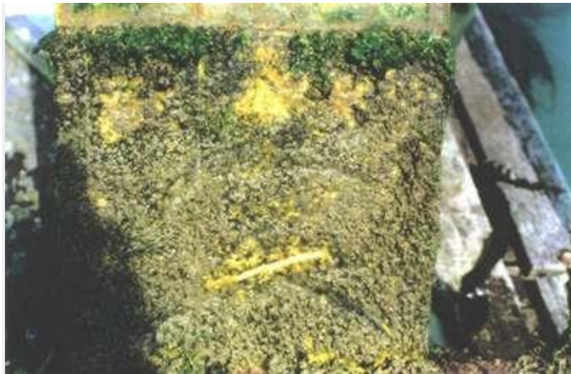
FIGURE 4. A Cu-Ni sheathed FRP test panel after nearly 3 years' exposure in Langstone Harbour (United Kingdom). Finger pressure was sufficient to remove biofouling off the panel surface revealing the original 90-10 Cu-Ni substrate.
