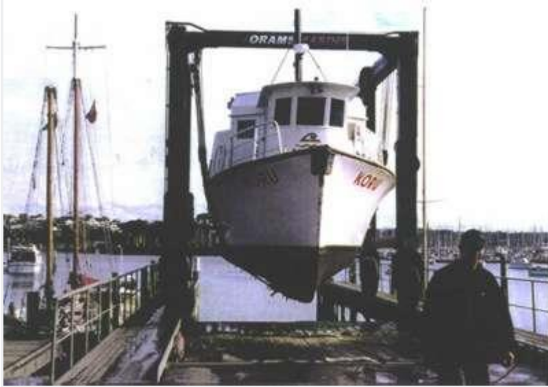
FIGURE 1. The ferry MV Koru , being hauled out of the harbour in Auckland. The vessel had last been hauled out one year previously. Note the relatively clean condition of the Cu-Ni sheathing after one year in seawater without cleaning.
