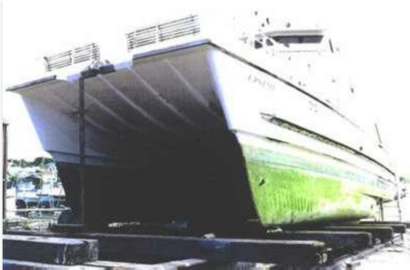
FIGURE 2. The catamaran ferry MV Osprey , being hauled out after one year's continuous service. Note that only slight microfouling (green algae) is visible where the hull is exposed to sunlight on the exterior surface of the nearest pontoon
