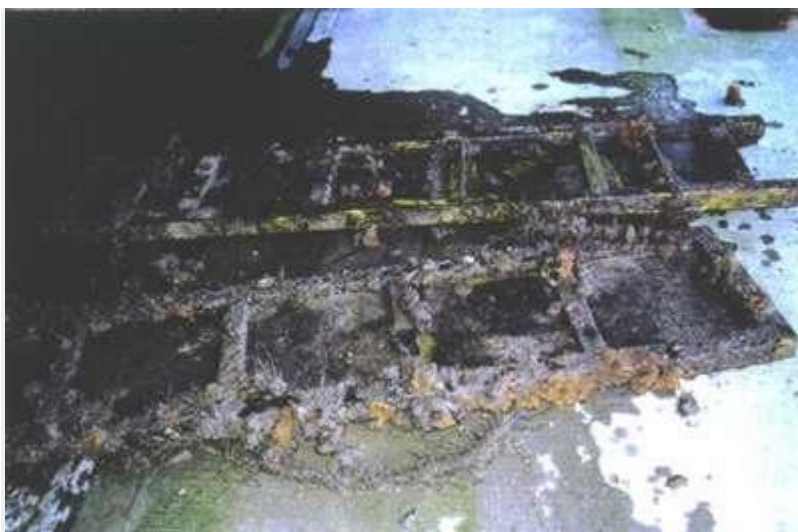
FIGURE 3. Two test panel frames removed after five years' seawater immersion at the Maritime Museum site, Auckland harbour, NZ. The differing degrees of fouling on the wooden frames are visible. The nearer wooden frame (steel panels) is painted, whilst the farther frame (aluminium panels) is clad with 90-10 Cu-Ni foil.
