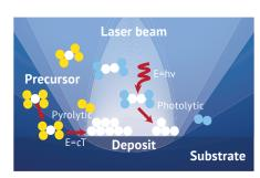
Figure 5 Laser beam guided selective area deposition from vapor phase metal precursor
