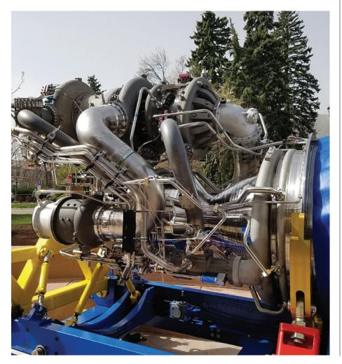
Far left: The housing of the Blue Origin BE-4 Ox Boost Pump is a single printed aluminum part and all of the stages of the hydraulic turbine are printed from K-500.
