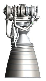
manufacturing approach allows the integration of complex internal flow passages in the housing that would be much more difficult to make using conventional methods. The turbine nozzles and rotors are also 3D printed
