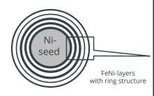
Figure 4 Layered structure of ferronickel pellets (dark color=Ni-rich, light color=iron-rich)
