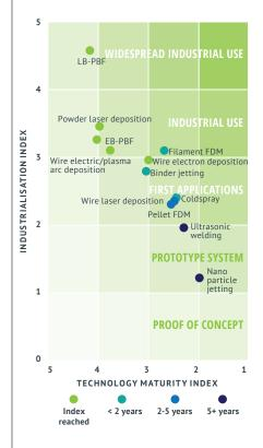
Figure 2 Technology and industrial maturity index of different Metal AM technologies
