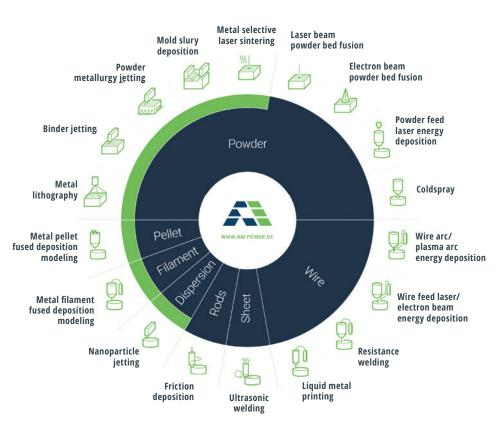
Figure 3 **Technology overview Metal Additive Manufacturing** Over 18 different metal 3D
