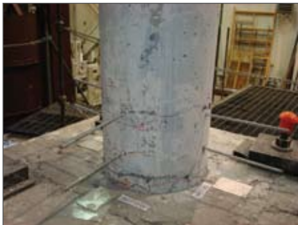
Minor damage in SMA/fibre concrete end
