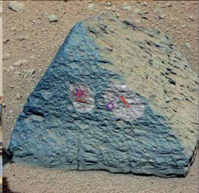
△ Above Right: The nickel-bearing Jake Matijevic rock. Red dots indicate laser targets, the circles show areas examined by the Alpha Particle X-Ray Spectrometer.
