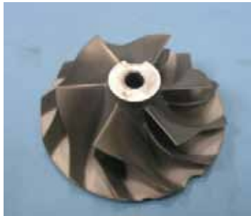
△ Above left: Compressor wheel with a nickel-phosphorus coating that allows engines to be efficient and low-emission for 500,000 km or more.
