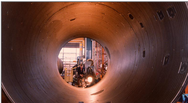
FIGURE 6. A view of the inside of a 3.5m diameter separator, 14m long, after electroslag cladding with Alloy 625.
