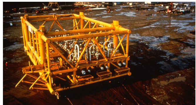
FIGURE 14. Subsea manifold (6" diameter piping) made of centricast clad pipe (X52 with 3mm Alloy 625 clad layer) for a North Sea project.
